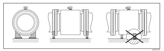
Fig. 14: Correct support for large nominal diameters (DN  $\geq$  350 / 14")
