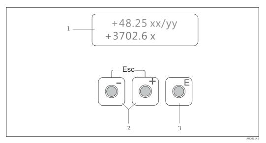
Fig. 48: Display and operating elements
