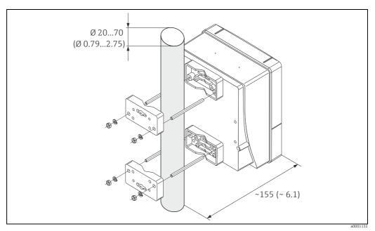
Fig. 30: Pipe mounting (wall-mount housing)
