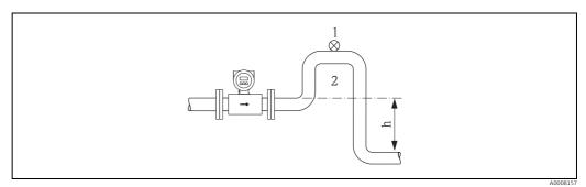
Fig. 9: Measures for installation in a down pipe
