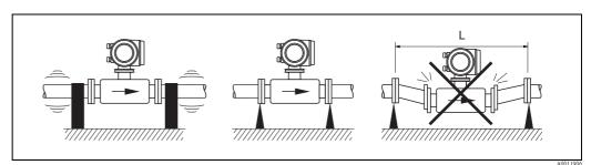
Measures to prevent vibration of the measuring device
