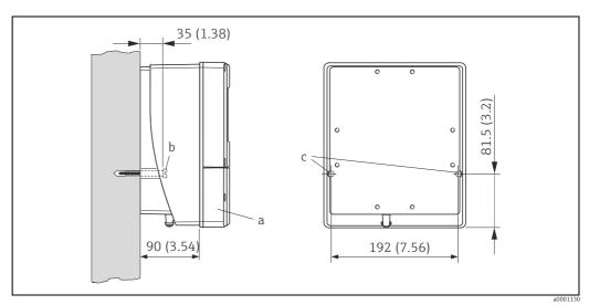
Fig. 28: Mounted directly on the wall
