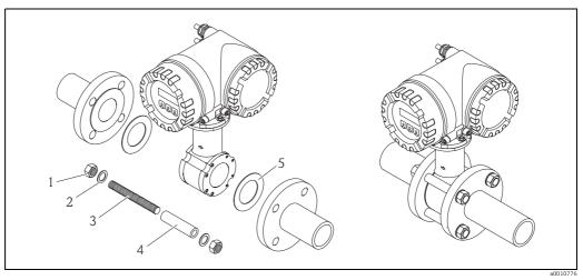
Fig. 17: Mounting the sensor
