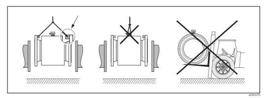
Fig. 5: Transporting sensors with DN > 300 (12")
