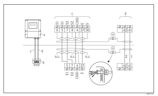
Fig. 33: Connecting the remote version of Promag  $\boldsymbol{H}$
