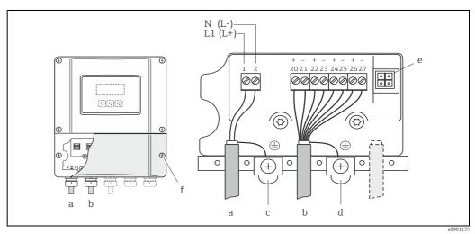
Fig. 37: Connecting the transmitter (wall-mount housing); cable cross-section: max. 2.5 mm<sup>2</sup>
