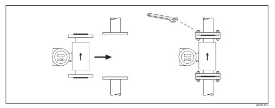
Fig. 24: Installing the Promag W sensor
