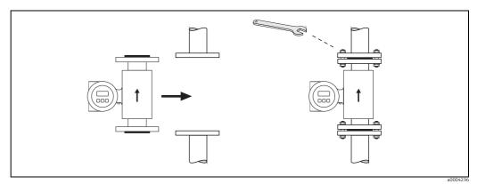
Fig. 18: Installing the Promag E sensor
