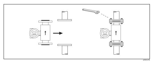
Fig. 21: Installing the Promag L sensor
