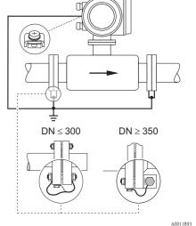
Via the ground terminal of the transmitter and the flanges of the pipe
