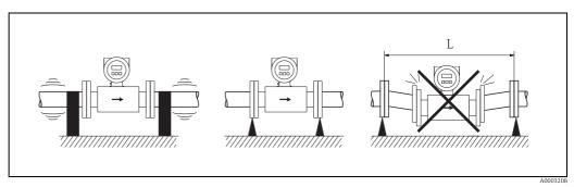
Fig. 13: Measures to prevent vibration of the device (L > 10 m (32.8 ft))
