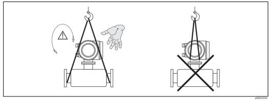
Fig. 4: Transporting sensors with DN  $\leq$  300 (12")
