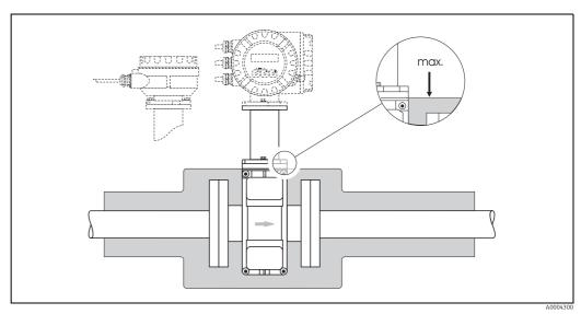
Fig. 23: Promag P (high-temperature version): Insulating the pipe
