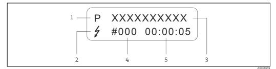
Fig. 50: Error messages on the display (example)
