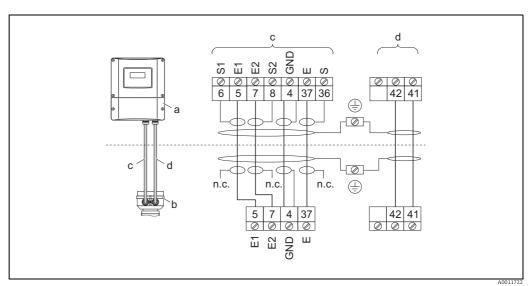
Fig. 32: Connecting the remote version of Promag E/L/P/W
