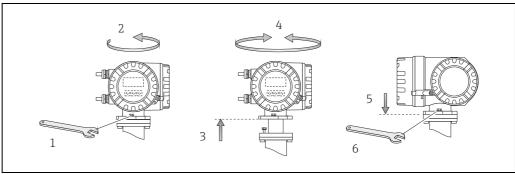
Fig. 25: Turning the transmitter housing (aluminum field housing)
