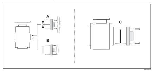
Promag H process connections (DN 2 to 25 / 1/12 to 1", DN 40 to 100 / 1½ to 4") Abb. 19:
