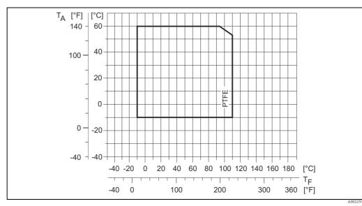
*Fig.* 59: Compact and remote version Promag E (TA = ambient temperature; TF = fluid temperature)
