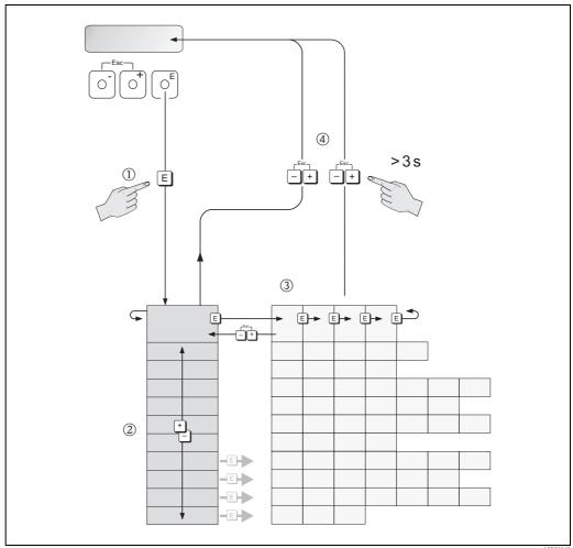
Selecting functions and configuring parameters (function matrix)
