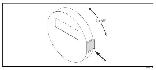
Fig. 27: Turning the local display (field housing)
