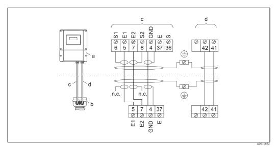
Fig. 31: Connecting the remote version of Promag D
