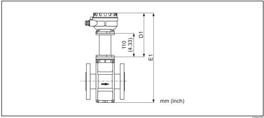
Measurement D1, E1 = Measurement D, E of the standard remote version plus 110 mm (4.33")
