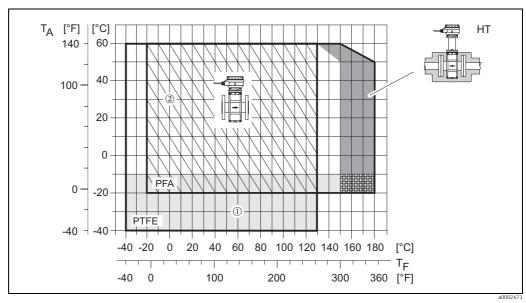
Abb. 61: Remote version Promag P (with PFA- or PTFE-lining)
