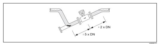
Fig. 8: Installation in a partially filled pipe
