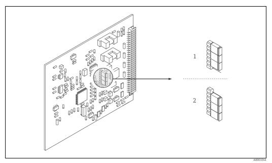
Fig. 52: Configuring current outputs using jumpers (I/O board)
