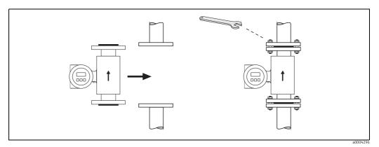
Fig. 22: Installing the Promag P sensor
