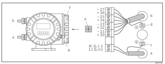
Fig. 35: Connecting the transmitter (aluminum field housing). Cable cross-section: max. 2.5 mm<sup>2</sup>
