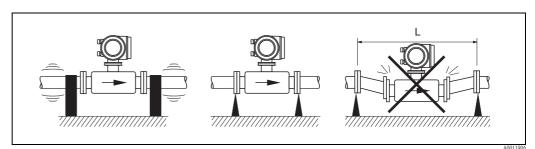
Measures to prevent vibration of the measuring device
