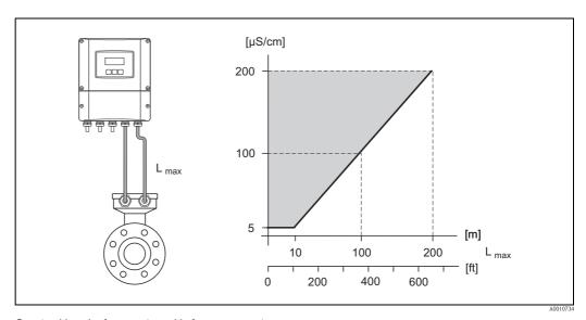
Permitted length of connecting cable for remote version Area marked in gray = permitted range;  $L_{max}$  = length of connecting cable in [m] ([ft]); fluid conductivity in [ $\mu$ S/cm]
