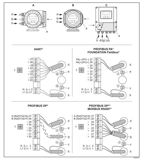
Connecting the transmitter, cable cross-section max. 2.5 mm<sup>2</sup> (14 AWG)
