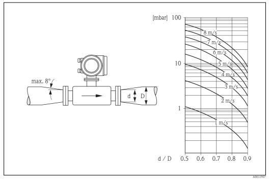
Fig. 15: Pressure loss due to adapters
