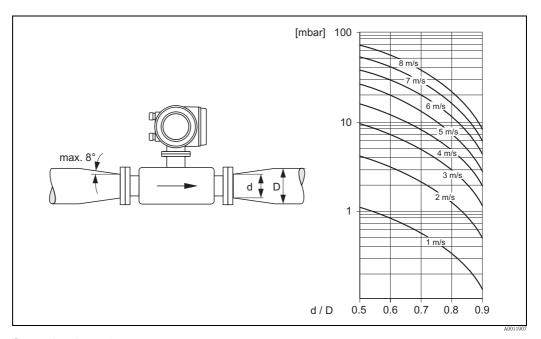
Pressure loss due to adapters
