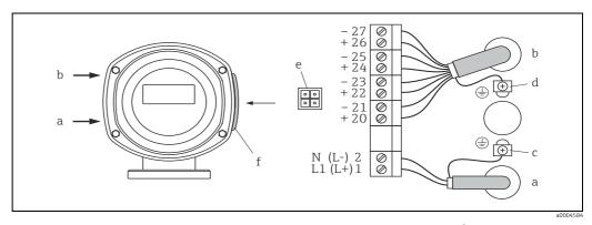
Fig. 36: Connecting the transmitter (stainless steel field housing); cable cross-section: max. 2.5 mm<sup>2</sup>
