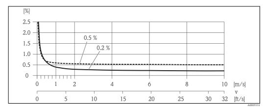
Fig. 58: Max. measured error in % of reading
