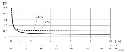
Max. measured error in % of reading
