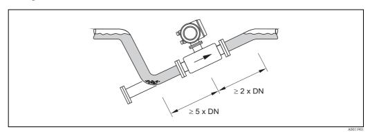
Installation with partially filled pipes
