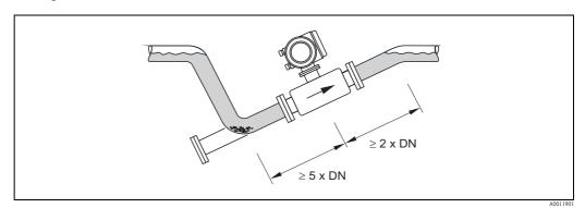
Installation with partially filled pipes
