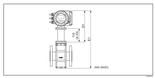
Measurement D1, E1 = Measurement D, E of the standard compact version plus 110 mm (4.33")
