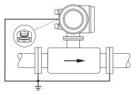
Via the ground terminal of the transmitter and the optionally available ground disks
