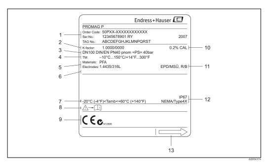
Fig. 2: Nameplate specifications for the "Promag" sensor (example)
