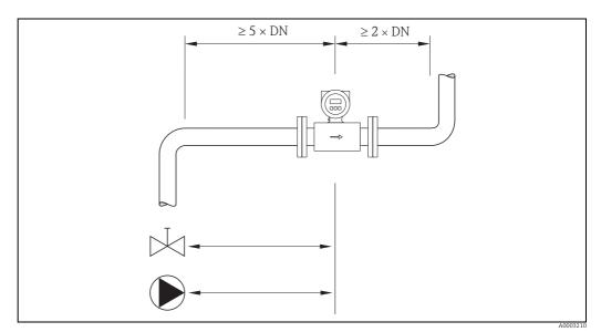
Fig. 12: Inlet and outlet runs
