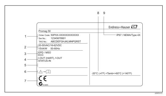
Nameplate specifications for the "Promag 50" transmitter (example) Fig. 1:
