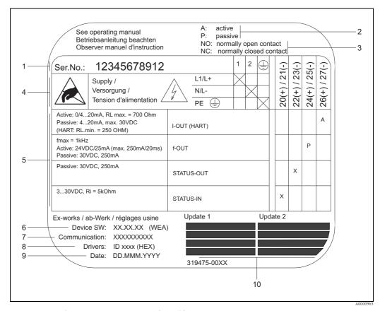
Fig. 3: Nameplate specifications for transmitter (example)
