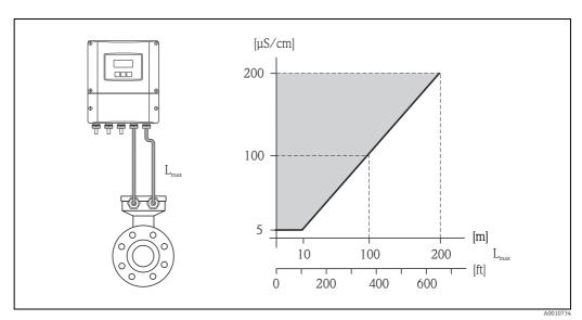
Fig. 16: Permissible cable length for the remote version
