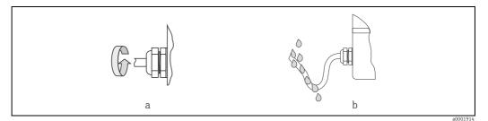
Fig. 47: Installation instructions, cable entries
