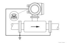
Potential equalization and cathodic protection
