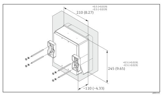
Fig. 29: Panel installation (wall-mount housing)
