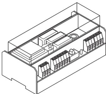
DigiTrace power-line carrier interfaces (PLI) modules provide temperature-monitoring capability for the DigiTrace NGC-30 heat-tracing control and monitoring unit. The PLI receives input from the power wires for the heat-tracing circuits, which carry the signals from special transmitters. The transmitters provide pipe temperatures from RTDs and continuity confirmation; they are typically located at the unpowered end of the heat-tracing line.
