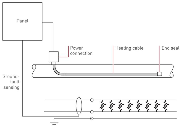
**Fig. 3 Ground-fault monitoring of actual G-F current**
