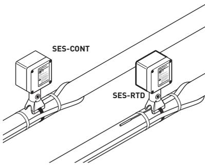
The SES series of transmitters is used in conjunction with the DigiTrace PLI and comes in two types: temperature/continuity transmitter (SES-RTD) and continuity transmitter (SES-CONT). These transmitters are used in freeze protection and process temperature maintenance applications. The system is unique in that the heating cable bus wires and power cables carry the monitoring signals. No additional field wire is necessary.
