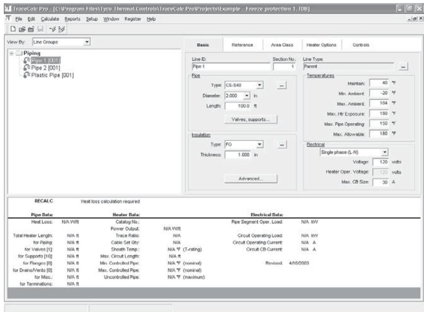
Fig. 1 TraceCalc Pro heat-tracing design software
