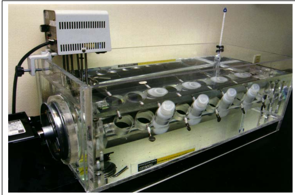
In vitro extraction apparatus used to conduct bioaccessibility testing of soils
